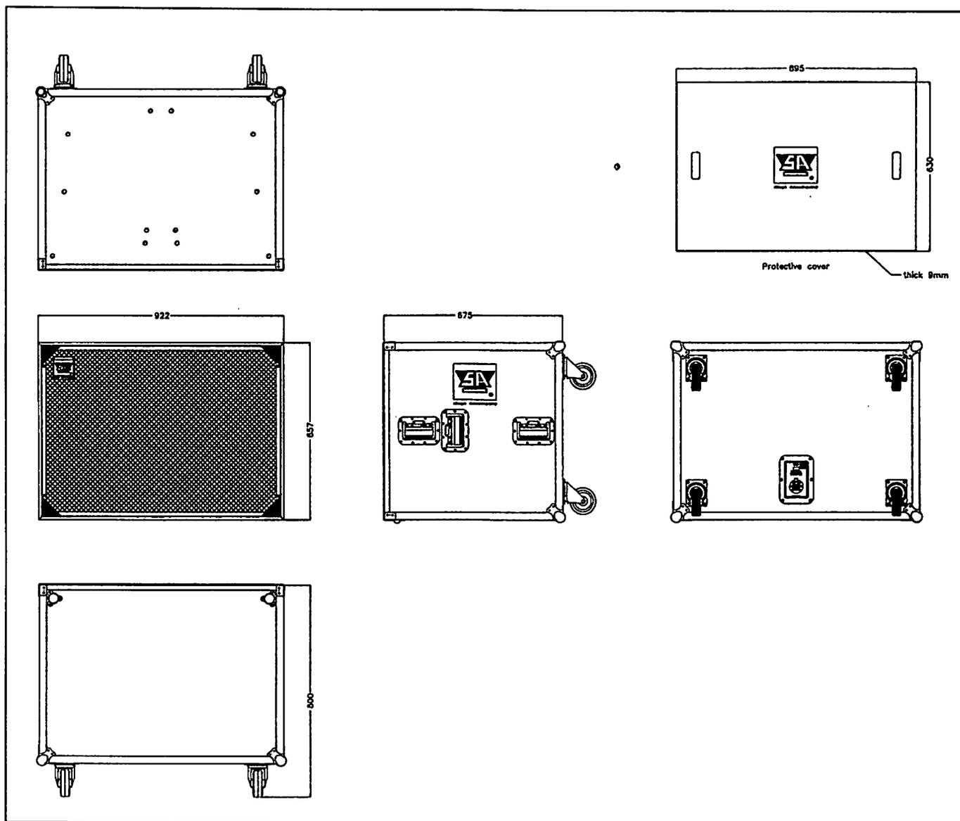
Physical dimensions of the SA 4817; flightcased version. The protective cover for transportation is shown in the upper right corner.
