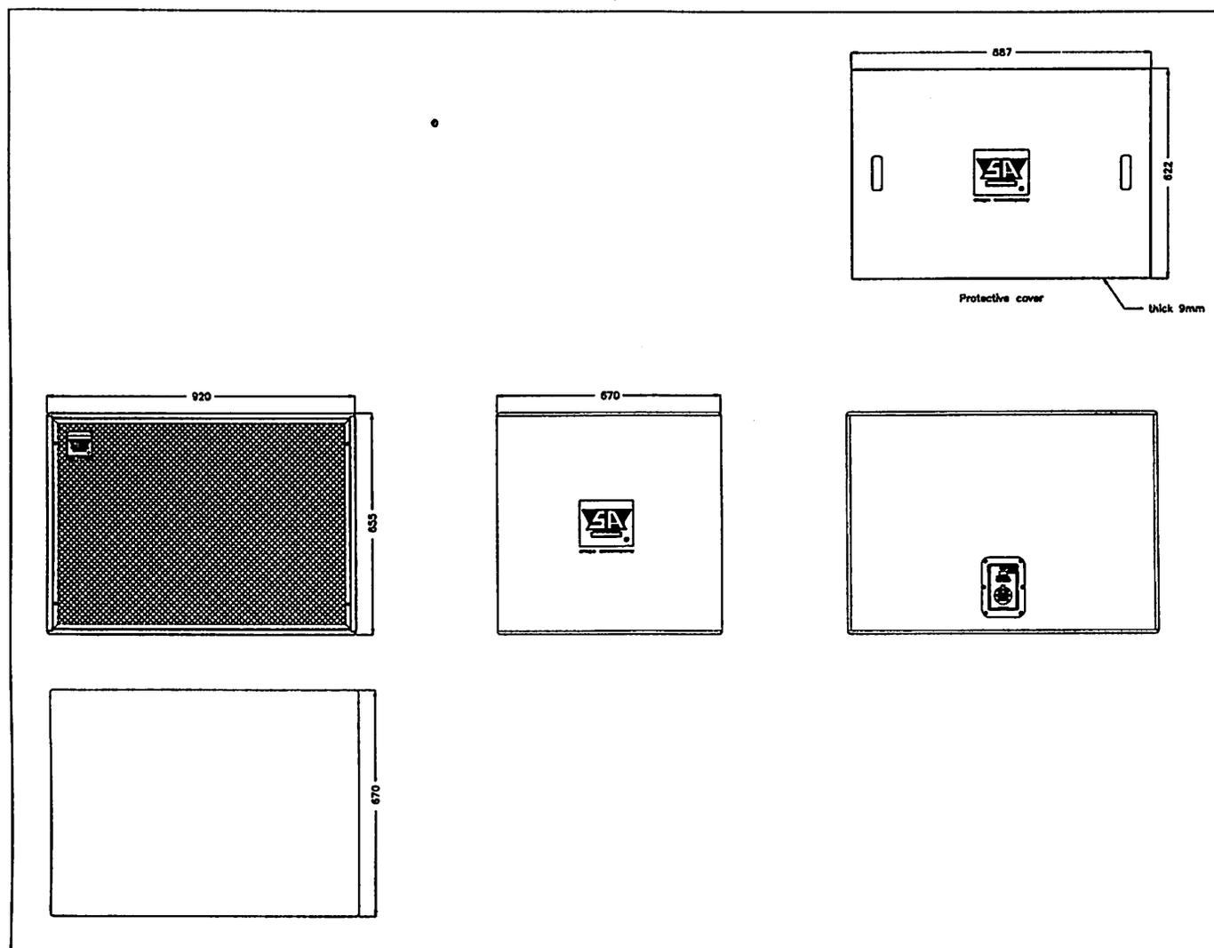
Physical dimensions of the SA 4817; normal version. The protective cover for transportation is shown in the upper right corner.
