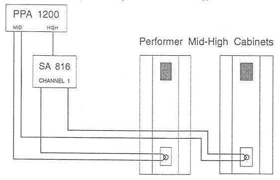
The SA 816 can be delivered with 2, 4, 6 or 8 channels (for 4, 8, 12 or 16 mid/high cabinets) depending on the job.
