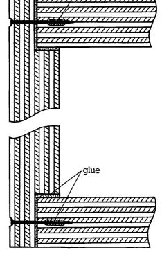
The "tongue-and-groove" construction gives better panel support and increased useful area where glue joints the panels. Special machine-injected nails are covered with glue that melts during injection to prevent them from disengaging.
