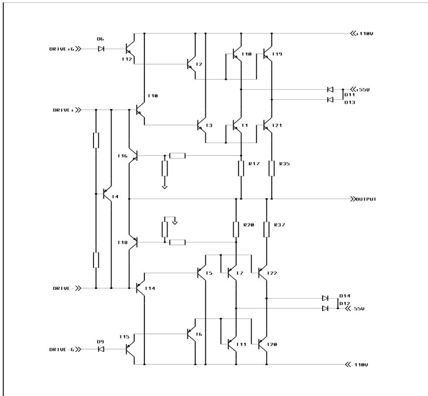
Figure 3.2 ES10 power amplifier set-up.
