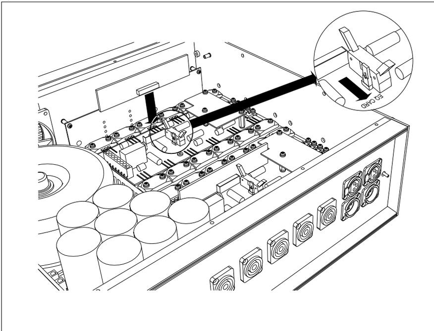
fig 6.1 Installing the EFN board for channel 1.
